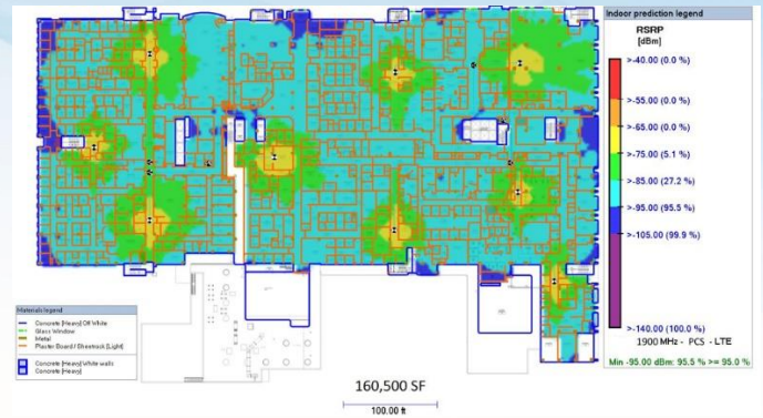
Figure 8. Wall type Sheet rock-Light (incorrect Passing)
